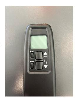
• The "send" symbol appears in the top left corner of the display when either of the two large buttons is pressed.
